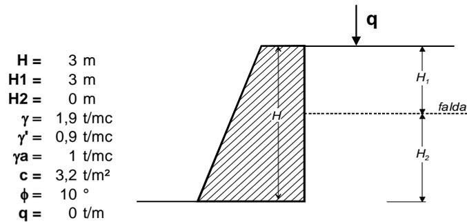
$$P_A = \frac{1}{2} K_a (\gamma H_1^2 + \gamma' H_2^2 + 2\gamma H_1 H_2) - \frac{2cH}{\sqrt{K_p}} + \frac{\gamma_d H_2^2}{2} + qK_a$$
